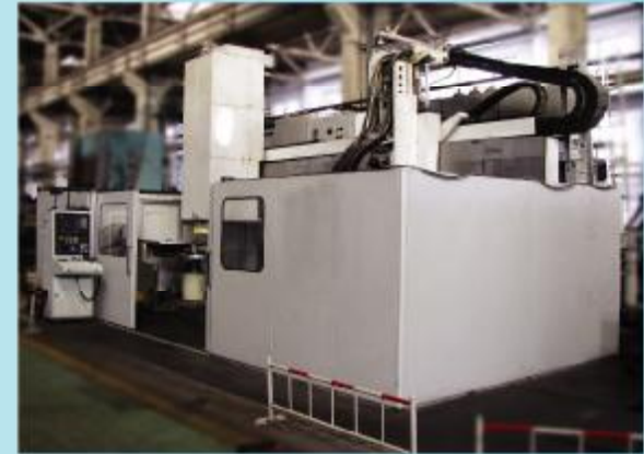
引进的进口大型磨床，可以加工 2.8 米外径，精度可以控制在 0.005mm 以内 The introduction of large-scale import grinder, can be processed outside diameter 2.8 meters, precision can be controlled within 0.005mm
